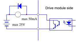
Fig. 3-8 Type2 switch value output interface
