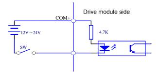
Fig. 3-7 Type1 switch value input interface
