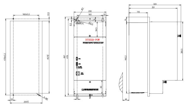
Fig. 2-1 The aperture dimension of DTS02A-POW
