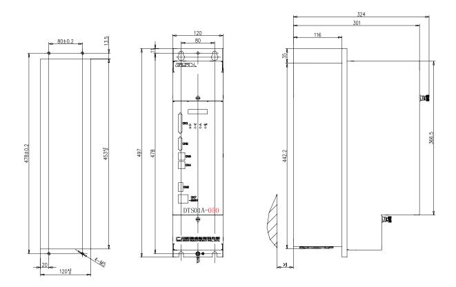
Fig. 2-1(b) The aperture dimension of DTS01A-05
