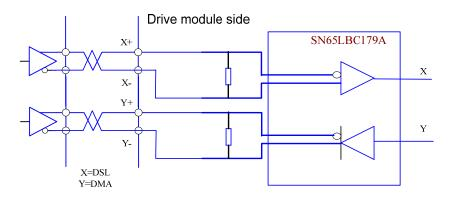
Fig. 3-11 Absolute photoelectricity encoder input interface
