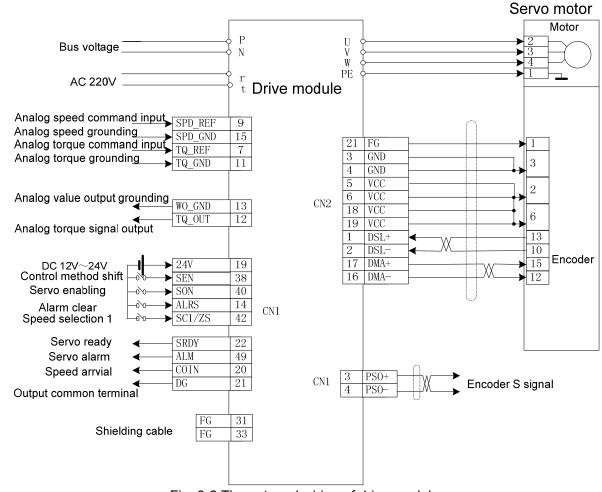
Fig. 3-2 The external wiring of drive module
