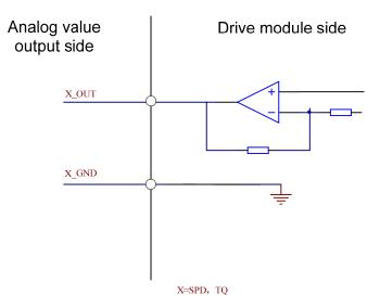
Fig. 3-10 Analog value output circuit
