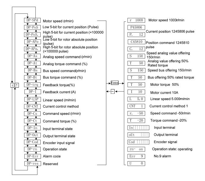
Fig. 6-2 The operation frame of monitoring method
