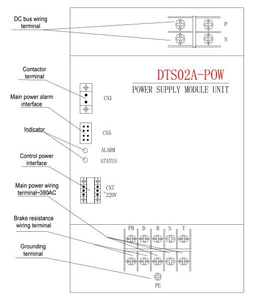
Fig. 1-1 The power module appearance of AE50 full electric injection molding machine specified drive unit
