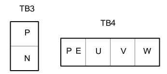
Fig. 3-3 The power terminal in drive unit
