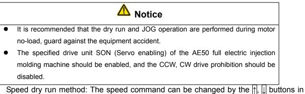
Speed dry run method: The speed command can be changed by the  $[\underline{1}]$ ,  $[\underline{1}]$  buttons in this method. The motor will operate based upon the supplied speed and direction. It is only used by the factory.
