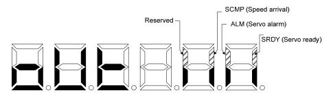
Fig. 6-4 Output terminal display (Stroke lights up that means ON, and vice versa)
