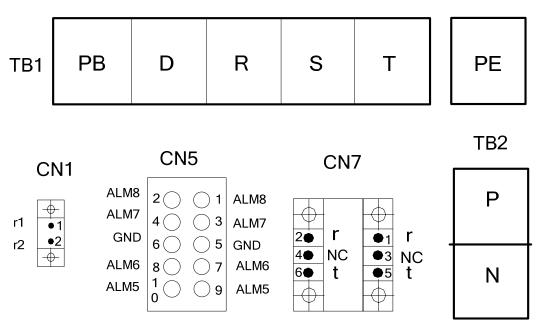
Fig. 3-1 DTS02A-POW terminal figure
