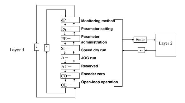
Fig. 6-1 Method operation frame
