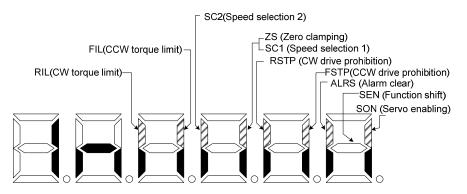
Fig. 6-3 Input terminal display (Stroke lights up that means ON, and vice versa)
