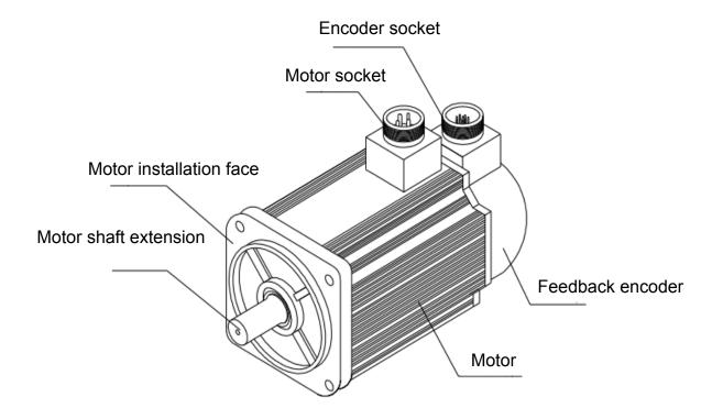
Fig. 1-3 SJT series servo motor appearance
